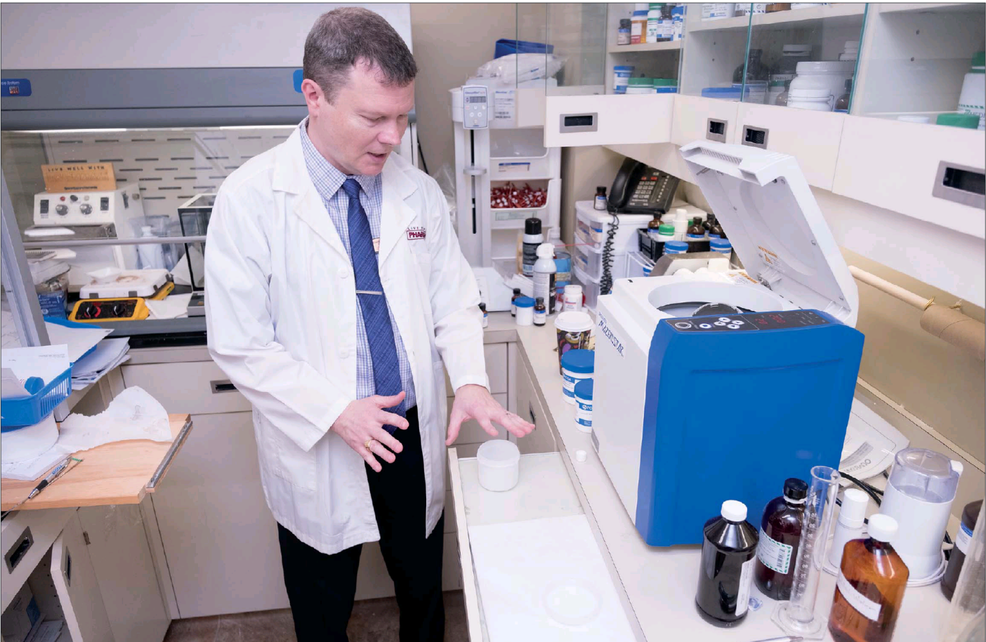
Pharmacist Graham Mackenzie in his compounding lab at Stone's Pharmasave in Baddeck - the only one of its kind in Cape Breton. His new compounding machine uses planetary motion to compound pain cream ingredients at 2000 revolutions per minute. Photo by Andrew Brooks.
